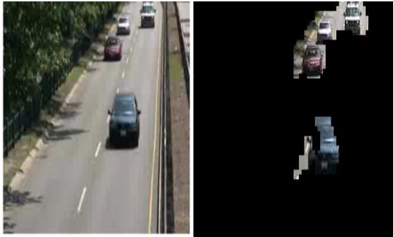
Fig 4.2: Input Frame, Final Segmentation.
